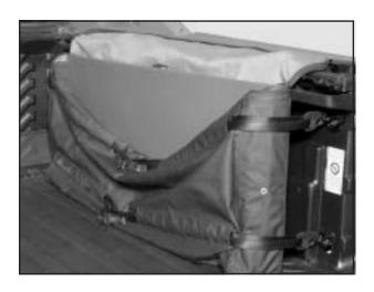
Starting with cargo panel 1, load the cargo panel with latches at the top of the bag and facing away from you.
